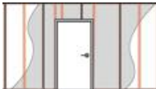
Forming door openings – front view.
