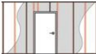
Forming door openings – front view.
